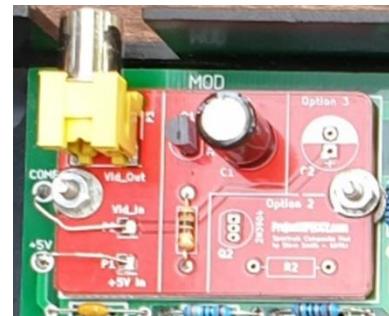
Spectrum 48K Composite Video Mod
